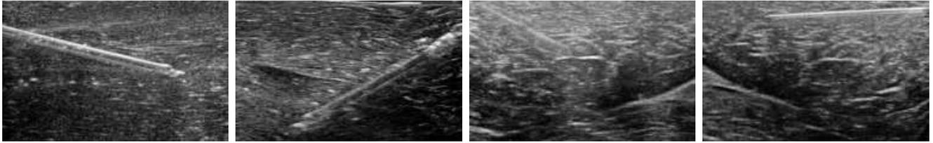
(a) Examples of needle detection in datasets of chicken breast phantom acquired with the 3D motorized linear array transducer.
