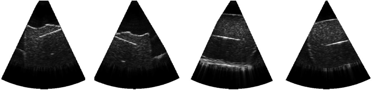
(b) Examples of needle detection in PVA cryogel phantom acquired with the 3D curved array transducer.
